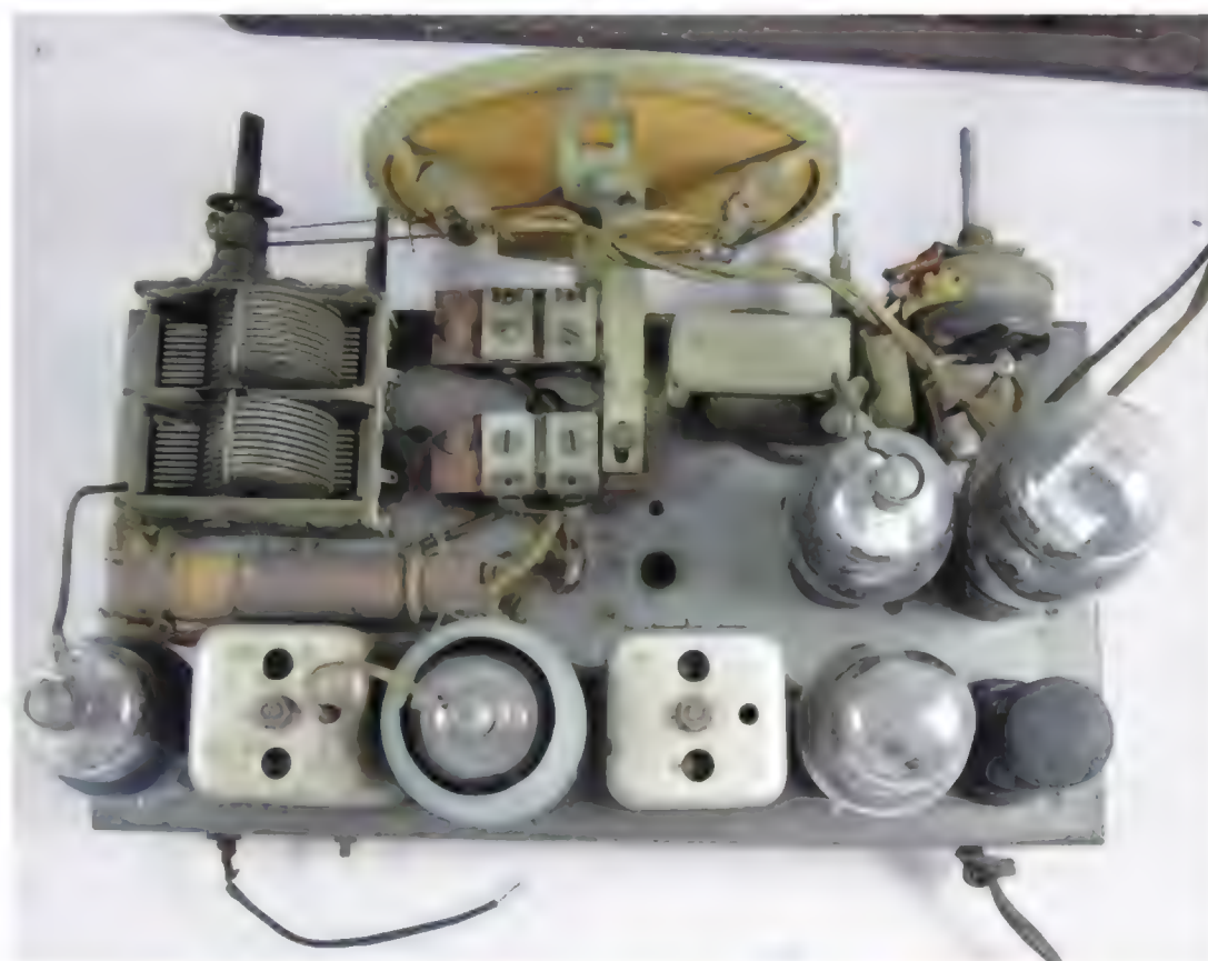
The DeWald 618 chassis from the top down.
